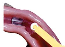
2. Insert the new plastic inserts with the yellow insertion tool (ref- 5021014). The plastic inserts will audibly click when they are inserted into the housing.
